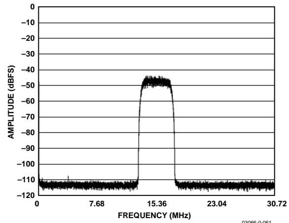
Figure 25. 32K FFT WCDMA Carrier @  $F_{IN} = 76.8$  MHz,
