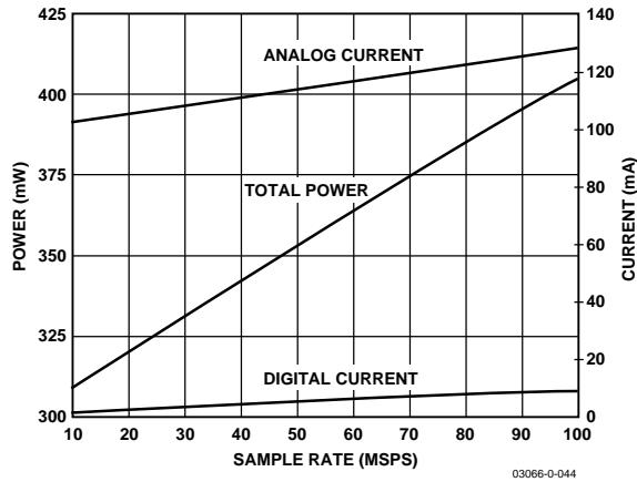
Figure 32. Power and Current vs. Sample Rate @ 2.5 MHz
