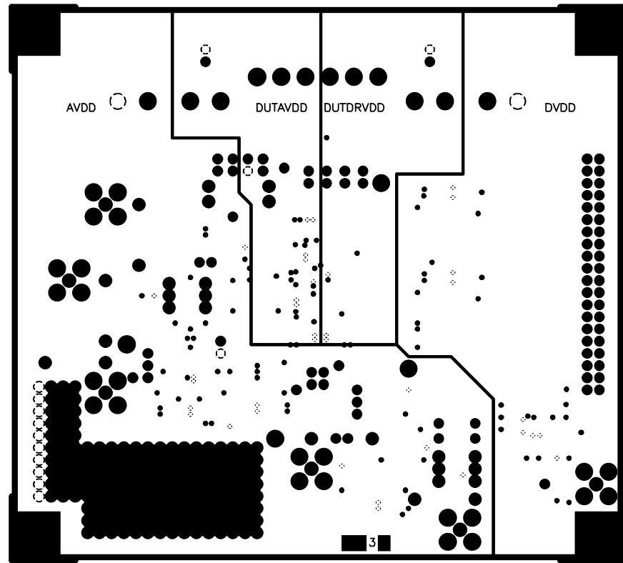
*Figure 45. TSSOP Evaluation Board Layout, Power Plane*
