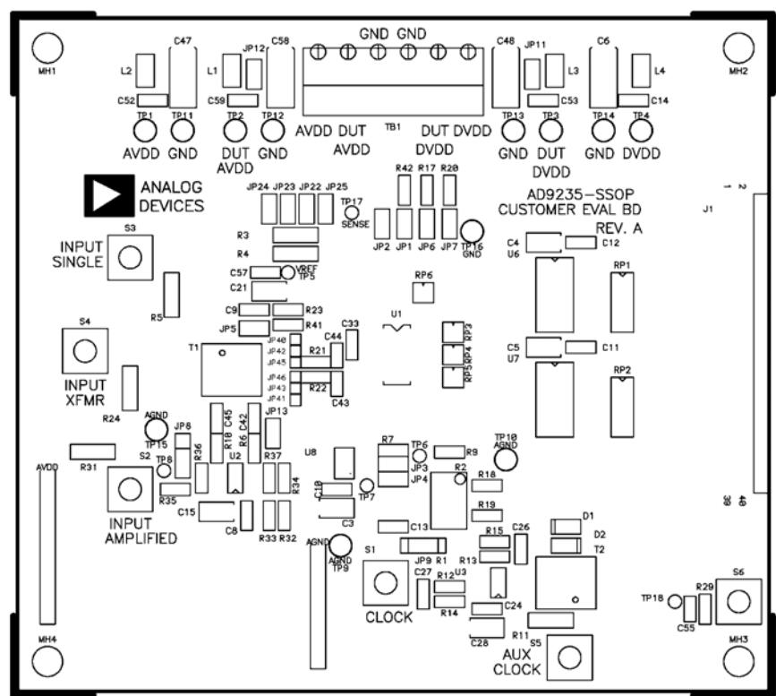
*Figure 46. TSSOP Evaluation Board Layout. Primary Silkscreen*
