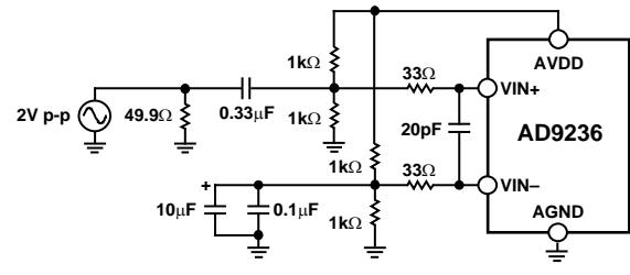
Figure 30. Single-Ended Input Configuration
