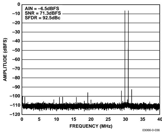
Figure 15. Two-Tone 8K FFT @ 30 MHz and 31 MHz
