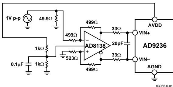
Figure 28. Differential Input Configuration Using the AD8138
