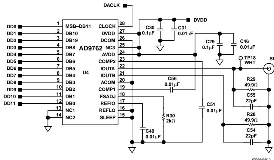
Figure 41. TSSOP Evaluation Board Schematic, Optional D/A Converter
