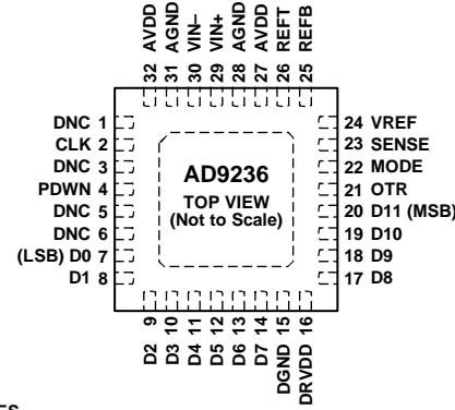
Figure 4. 32-Lead LFCSP
