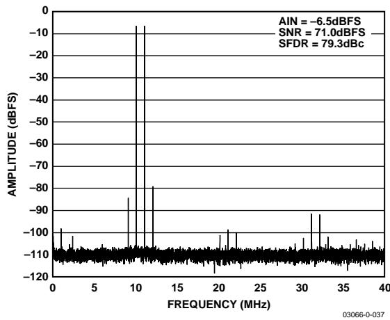
Figure 16. Two-Tone 8K FFT @ 69 MHz and 70 MHz
