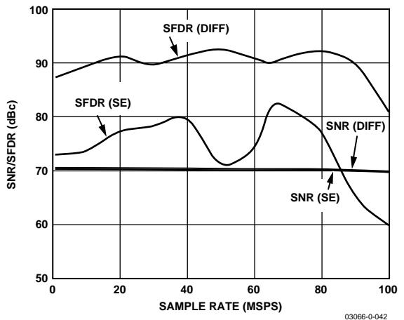
Figure 14. SNR/SFDR vs. Sample Rate @ 10 MHz
