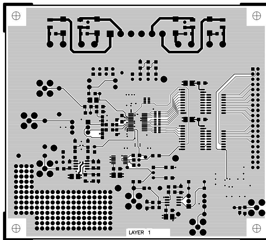
Figure 42. TSSOP Evaluation Board Layout, Primary Side
