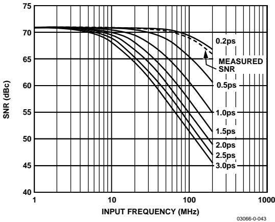
Figure 31. SNR vs. Input Frequency and Jitter
