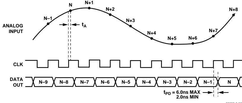
Figure 2. Timing Diagram
