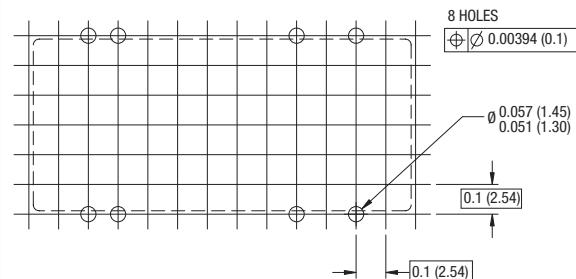
All dimensions in inches  $\pm 0.01$  (mm  $\pm 0.25$ mm). All pins on a 0.1 (2.54) pitch and within  $\pm 0.01$  (0.25) of true position.
