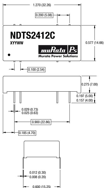
All dimensions in inches  $\pm 0.01$  (mm  $\pm 0.25$ mm). All pins on a 0.1 (2.54) pitch and within  $\pm 0.01$  (0.25) of true position.
