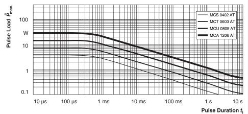
Maximum pulse load, single pulse; applicable if  $\bar{P} \to 0$  and  $n \le 1000$  and  $\hat{U} \le \hat{U}_{max}$ ; for permissible resistance change equivalent to 8000 h operation in standard operation mode **Single Pulse**
