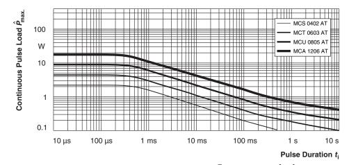
Maximum pulse load, continuous pulses; applicable if  $\overline{P} \leq P\left(\vartheta_{\text{amb}}\right)$  and  $\hat{U} \leq \hat{U}_{\text{max}}$ ; for permissible resistance change equivalent to 8000 h operation in standard operation mode
