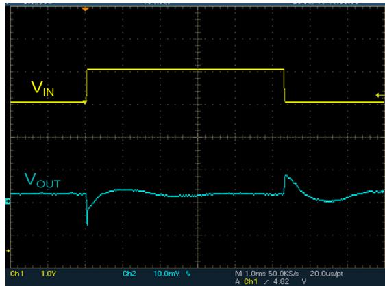
$V_{IN} = 5V$ ,  $V_{OUT}=3V$ ,  $I_{OUT}=0mA$ ,  $C_{OUT}=1\mu F$ ,  $\Delta V_{IN} = 500mV$
