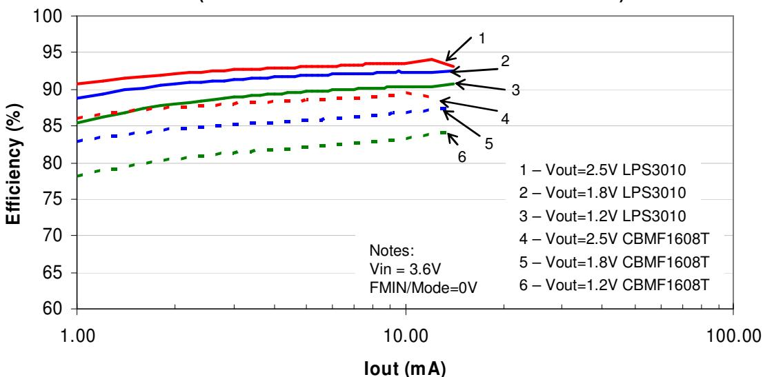
Figure 4. Typical Efficiency vs. Load Current for Different Inductors
