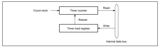
Figure 2.17 Example of Timer Configuration with Two Registers
