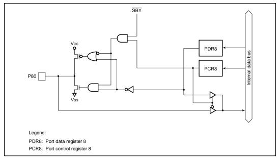
Figure B.6 Port 8 Block Diagram (Pin P80)
