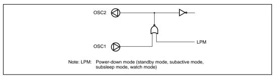
Figure 4.3 Block Diagram of System Clock Generator
