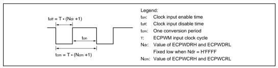
Figure 9.10 Event Counter Operation Waveform
