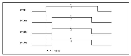
Figure 14.7 Timing for Operation/Release of Low-Voltage Detection Circuit
