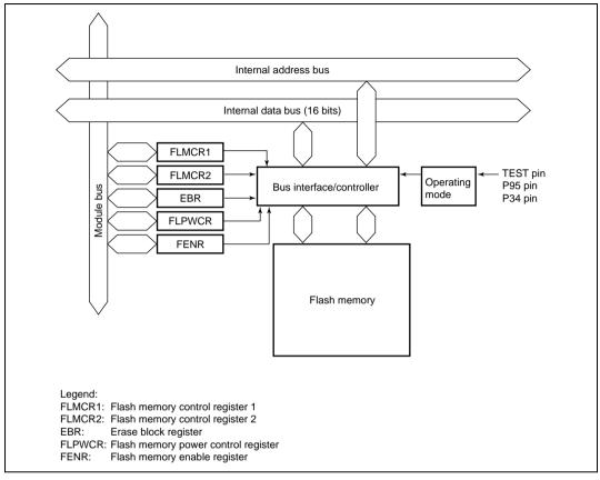
Figure 6.7 Block Diagram of Flash Memory
