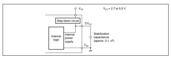
Figure 15.1 Power Supply Connection when Internal Step-Down Circuit is Used
