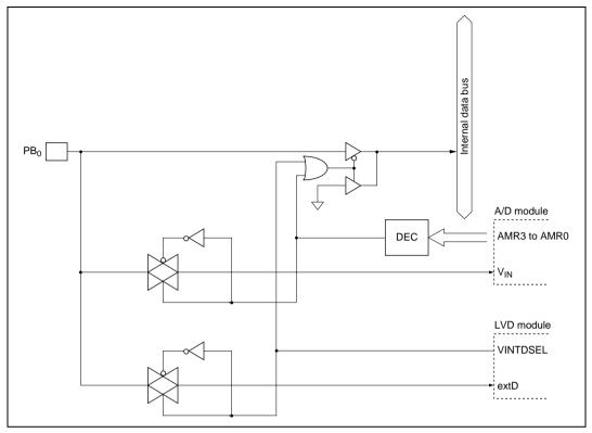
Figure B.9(b) Port B Block Diagram (Pin PB0, H8/38104 Group Only)
