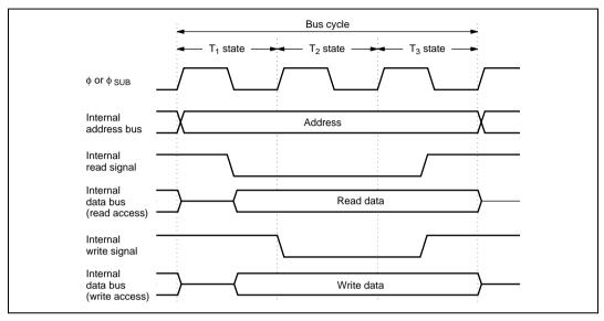
Figure 2.14 On-Chip Peripheral Module Access Cycle (3-State Access)
