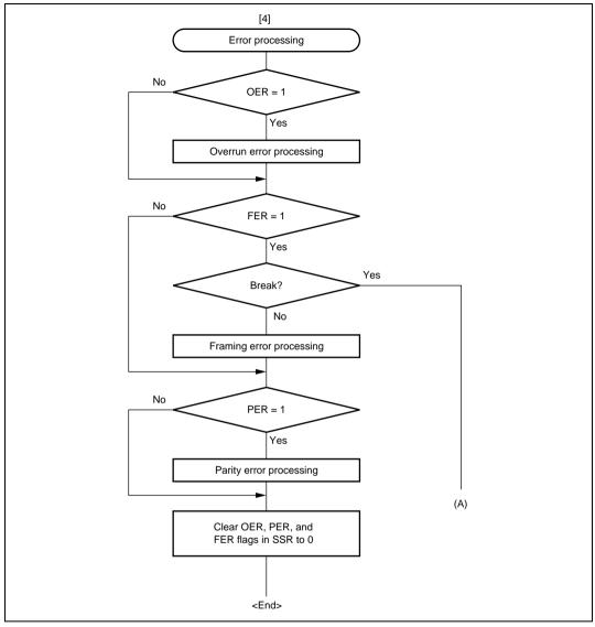
Figure 10.8 Sample Serial Data Reception Flowchart (Asynchronous Mode) (2)
