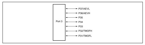
Figure 8.1 Port 3 Pin Configuration
