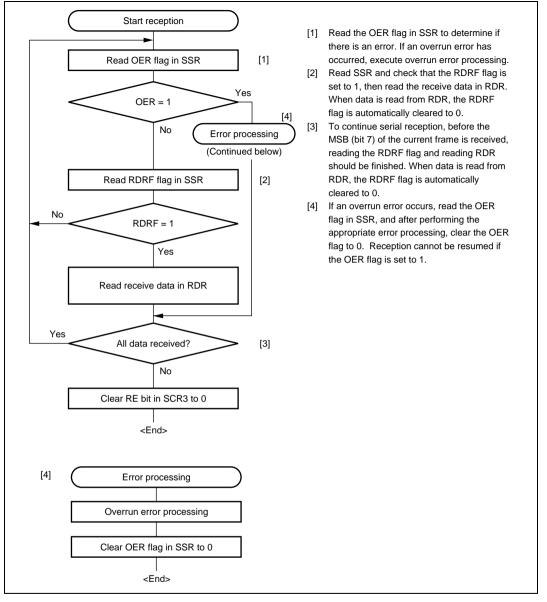
Figure 10.13 Sample Serial Reception Flowchart (Clocked Synchronous Mode)
