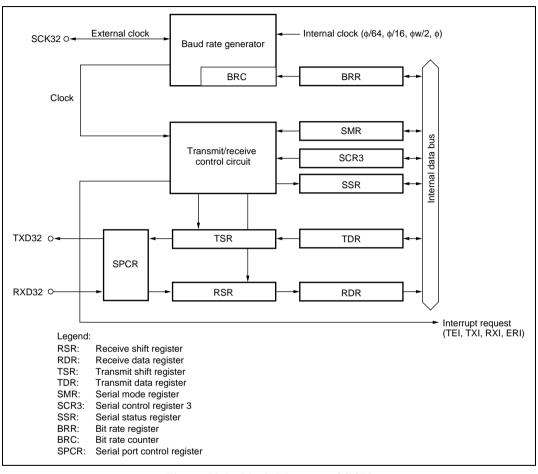
Figure 10.1 Block Diagram of SCI3
