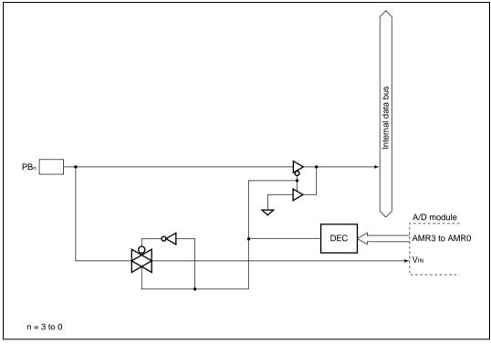
Figure B.9(a) Port B Block Diagram
