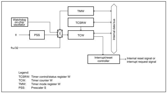
Figure 9.12(2) Block Diagram of Watchdog Timer (H8/38104 Group)
