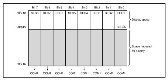
Figure 13.6 LCD RAM Map (Static Mode)
