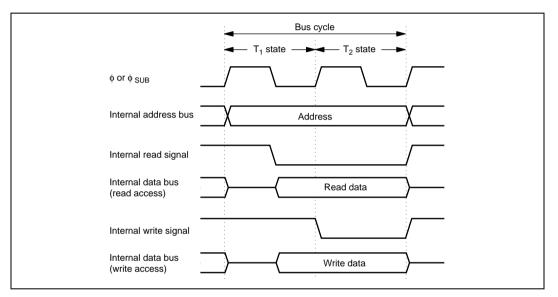
Figure 2.13 On-Chip Peripheral Module Access Cycle (2-State Access)
