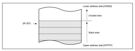
Figure 2.3 Stack Pointer
