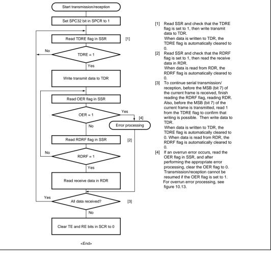
Figure 10.14 Sample Flowchart of Simultaneous Serial Transmit and Receive Operations (Clocked Synchronous Mode)
