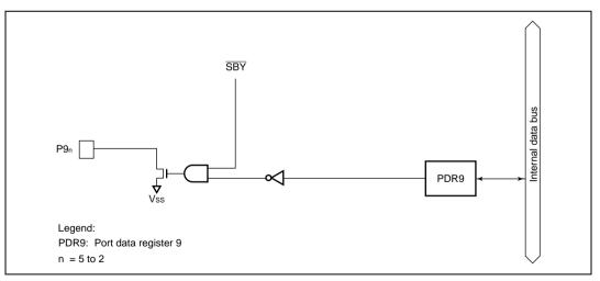
Figure B.7(b) Port 9 Block Diagram (Pins P95 to P92)
