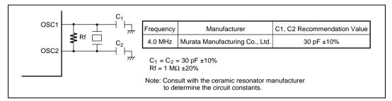
Figure 4.6(1) Typical Connection to Ceramic Resonator (H8/3802 Group)
