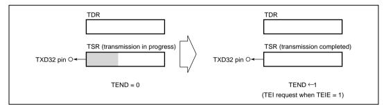
Figure 10.19(c) TEND Setting and TEI Interrupt
