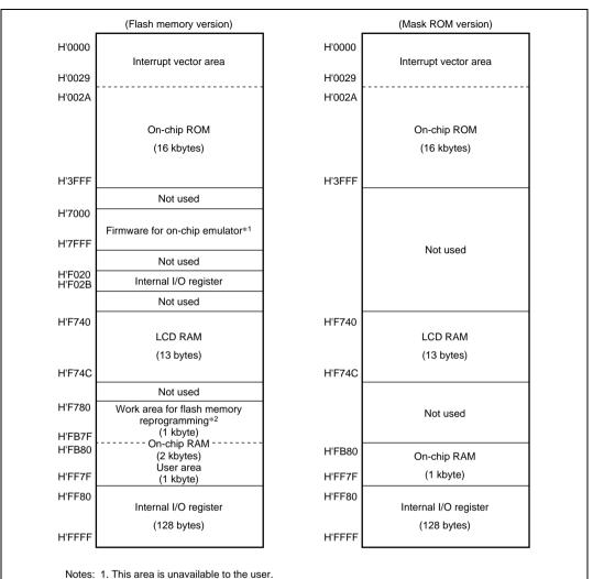
When flash memory is programmed, this area is used by the programming control program.When the on-chip emulator is used, this area is unavailable to the user.
