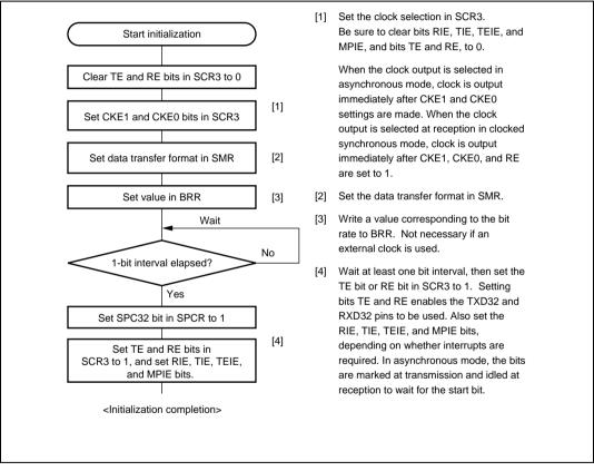
Figure 10.4 Sample SCI3 Initialization Flowchart
