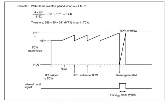
Figure 9.13 Example of Watchdog Timer Operation
