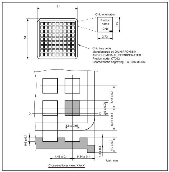
Figure H.2 Chip Tray Specifications (HCD64338004, HCD64338003, HCD64338002, HCD64338001, and HCD64338000)
