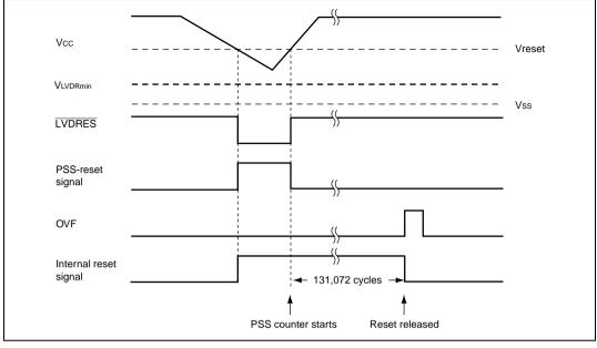
Figure 14.3 Operational Timing of LVDR Circuit
