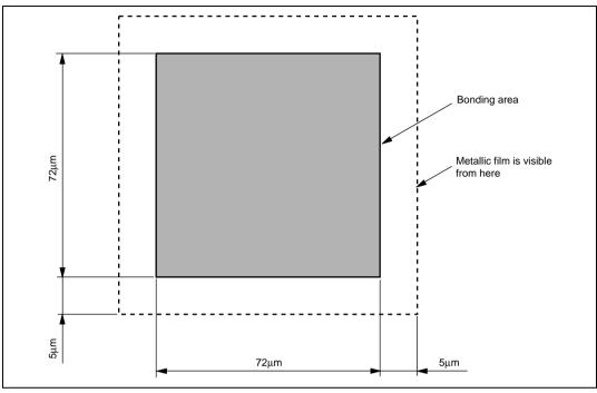
Figure G.1 Bonding Pad Form (HCD6433802, HCD6433801, HCD6433800, HCD64338004, HCD64338003, HCD64338002, HCD64338001, HCD64338000, HCD64F38004, and HCD64F38002)
