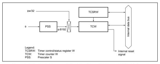
Figure 9.12(1) Block Diagram of Watchdog Timer (H8/38004, H8/38002S Group)
