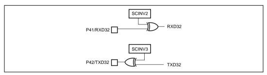
Figure 8.3 Input/Output Data Inversion Function
