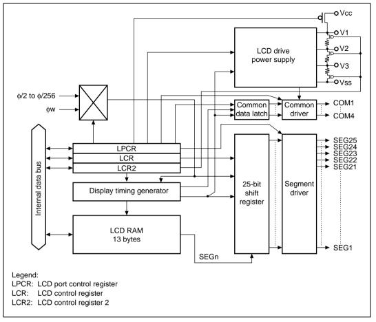
Figure 13.1(2) Block Diagram of LCD Controller/Driver (H8/38104 Group)
