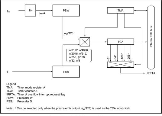
Figure 9.1 Block Diagram of Timer A
