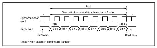
Figure 10.9 Data Format in Clocked Synchronous Communication
