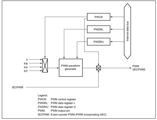
Figure 11.1(2) Block Diagram of 10-Bit PWM (H8/38104 Group)
