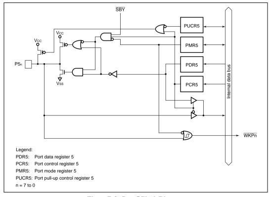
Figure B.3 Port 5 Block Diagram
