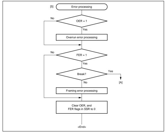
Figure 10.17 Sample Multiprocessor Serial Reception Flowchart (2)
