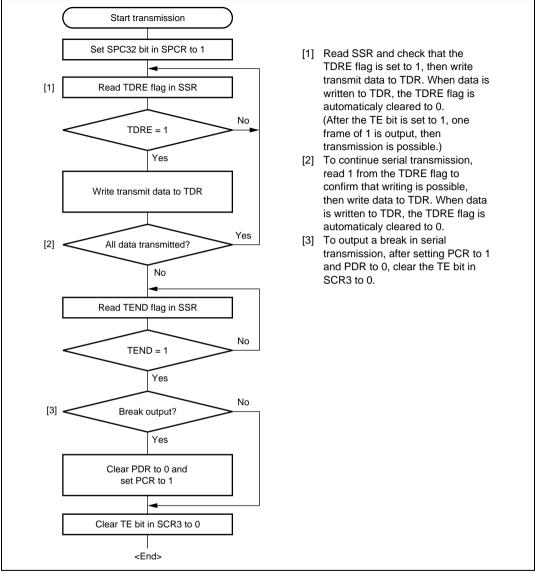
Figure 10.6 Sample Serial Transmission Flowchart (Asynchronous Mode)
