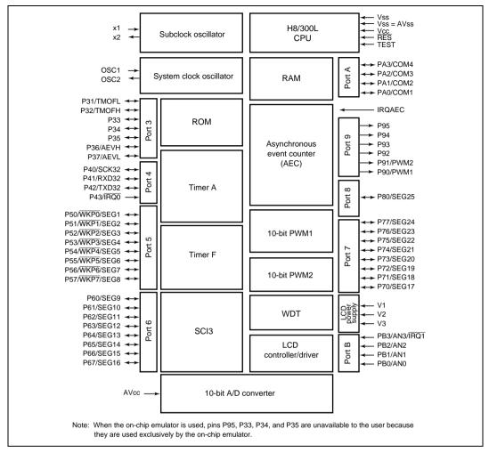
Figure 1.2 Internal Block Diagram of H8/38004 Group
