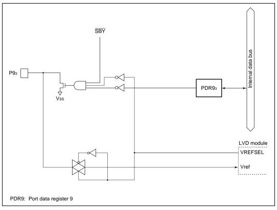
Figure B.7(c) Port 9 Block Diagram (Pin P93, H8/38104 Group Only)
