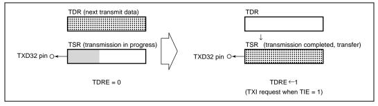
Figure 10.19(b) TDRE Setting and TXI Interrupt
