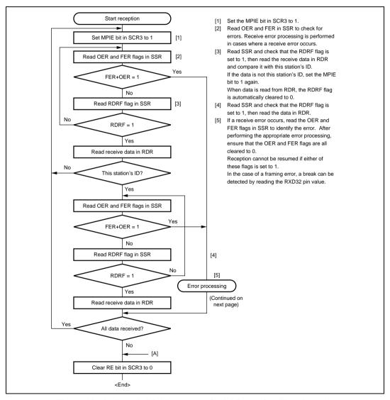
Figure 10.17 Sample Multiprocessor Serial Reception Flowchart (1)
