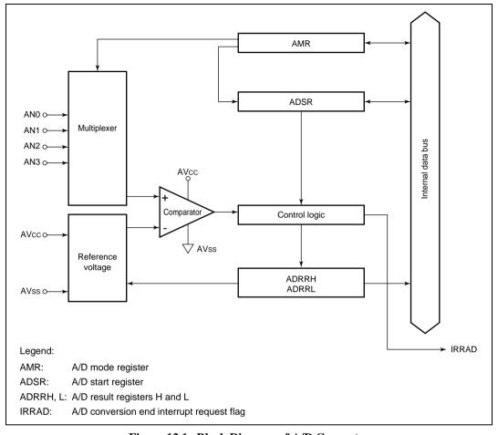
Figure 12.1 Block Diagram of A/D Converter
