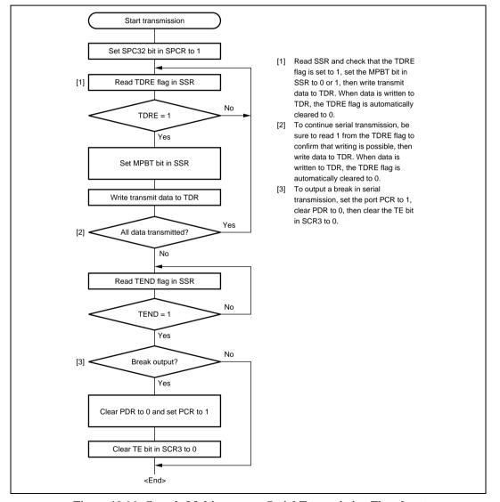
Figure 10.16 Sample Multiprocessor Serial Transmission Flowchart
