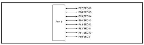
Figure 8.5 Port 6 Pin Configuration
