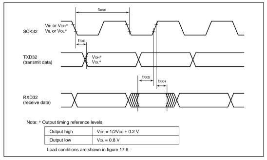
Figure 17.5 SCI3 Input/Output Timing in Clocked Synchronous Mode
