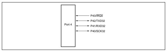
Figure 8.2 Port 4 Pin Configuration
