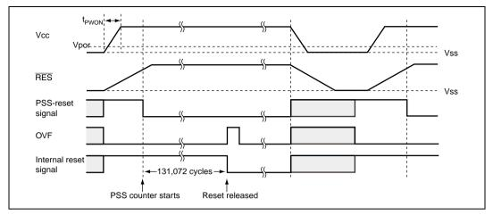
Figure 14.2 Operational Timing of Power-On Reset Circuit
