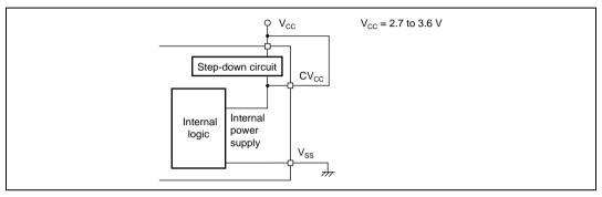
Figure 15.2 Power Supply Connection when Internal Step-Down Circuit is Not Used
