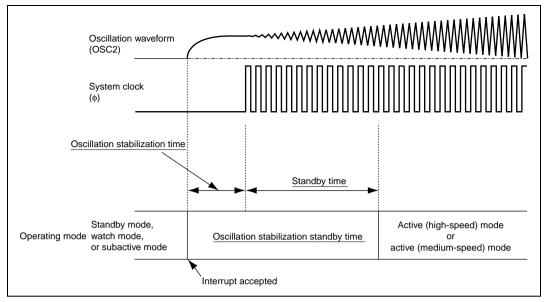
Figure 4.16 Oscillation Stabilization Standby Time
