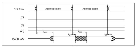
Figure 6.15 Timing Waveforms in  $\overline{\text{CE}}$  and  $\overline{\text{OE}}$  Enable State Read
