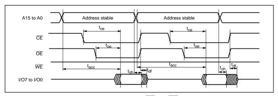
Figure 6.16 Timing Waveforms in  $\overline{\text{CE}}$  and  $\overline{\text{OE}}$  Clock System Read
