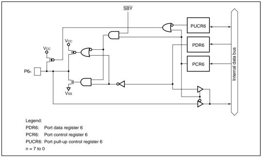
Figure B.4 Port 6 Block Diagram
