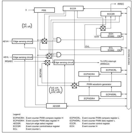
Figure 9.7 Block Diagram of Asynchronous Event Counter
