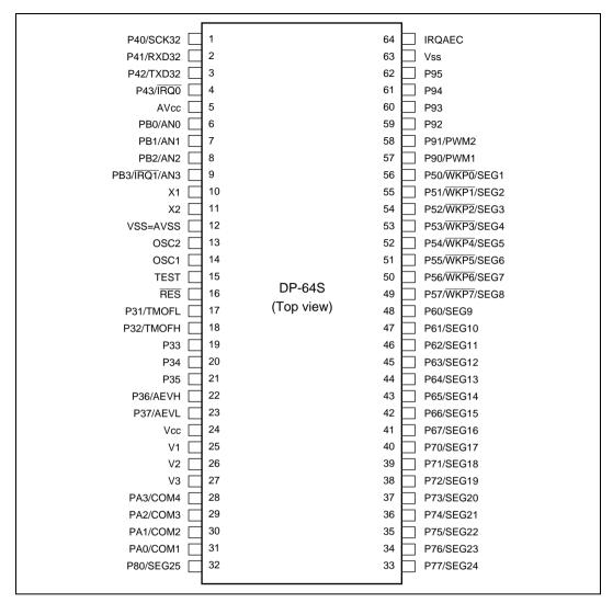
Figure 1.5 Pin Arrangement of H8/3802 Group (DP-64S)
