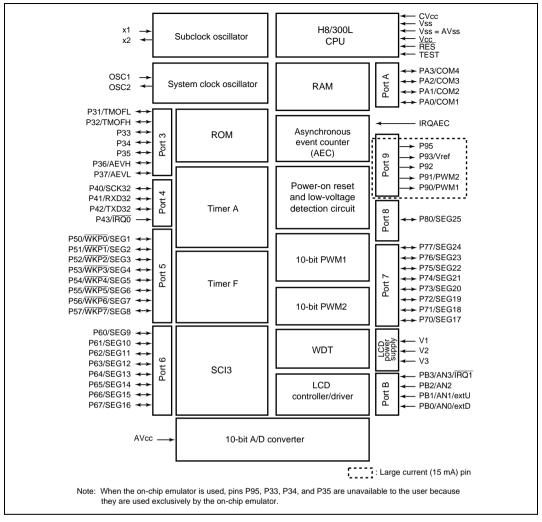
Figure 1.3 Internal Block Diagram of H8/38104 Group
