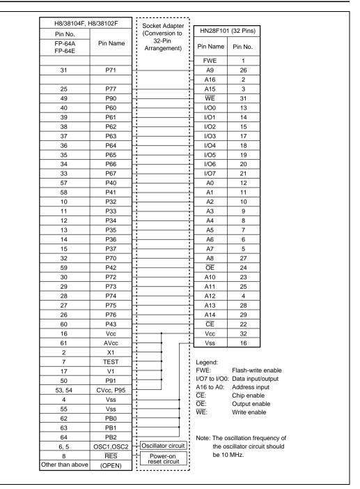
Figure 6.12(2) Socket Adapter Pin Correspondence Diagram (H8/38104F, H8/38102F)
