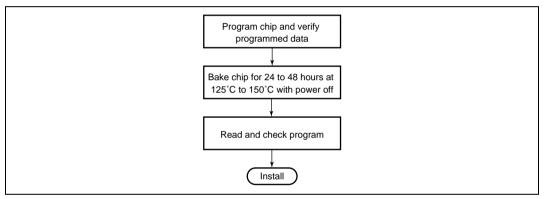
Figure 6.6 Recommended Screening Procedure
