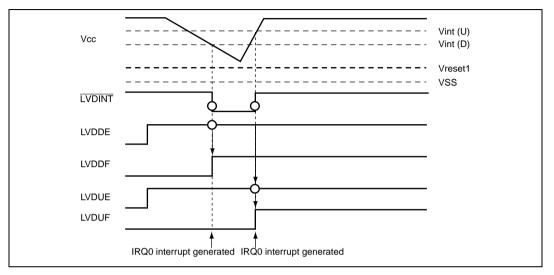
Figure 14.4 Operational Timing of LVDI Circuit
