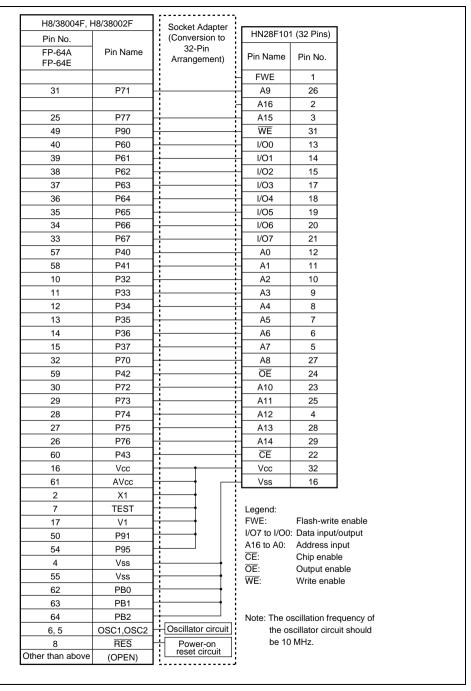
Figure 6.12(1) Socket Adapter Pin Correspondence Diagram (H8/38004F, H8/38002F)
