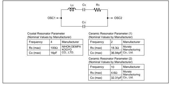
Figure 17.8 Resonator Equivalent Circuit
