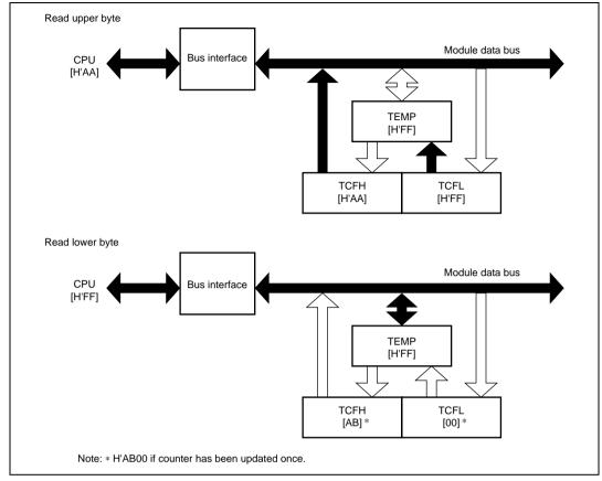
Figure 9.4 Read Access to TCF (TCF  $\rightarrow$  CPU)
