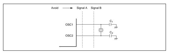
Figure 4.15 Example of Incorrect Board Design
