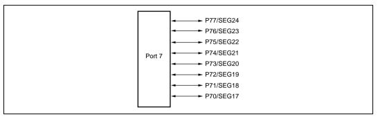
Figure 8.6 Port 7 Pin Configuration
