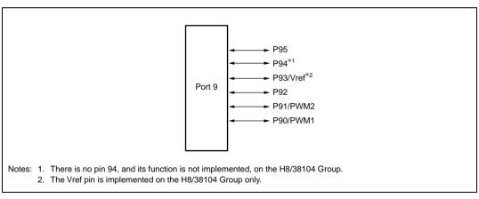
Figure 8.8 Port 9 Pin Configuration
