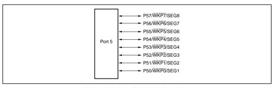
Figure 8.4 Port 5 Pin Configuration
