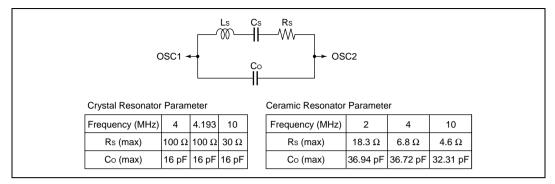
Figure 17.7 Resonator Equivalent Circuit
