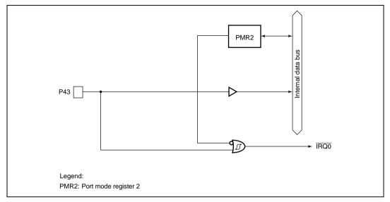
Figure B.2(a) Port 4 Block Diagram (Pin P43)
