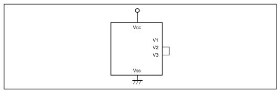
Figure 13.2 Handling of LCD Drive Power Supply when Using 1/2 Duty
