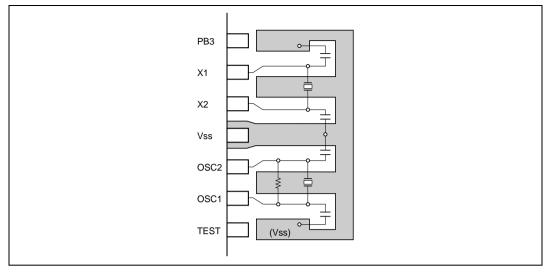
Figure 4.13 Example of Crystal and Ceramic Resonator Arrangement
