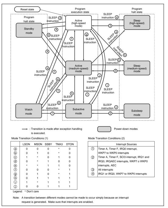
Figure 5.1 Mode Transition Diagram
