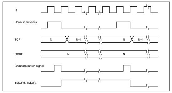
Figure 9.5 TMOFH/TMOFL Output Timing
