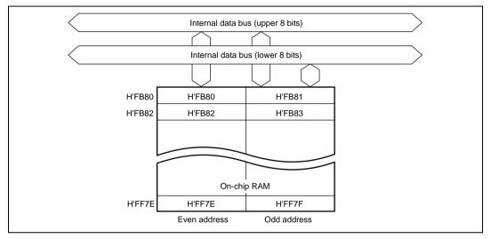
Figure 7.1 Block Diagram of RAM (H8/3802)
