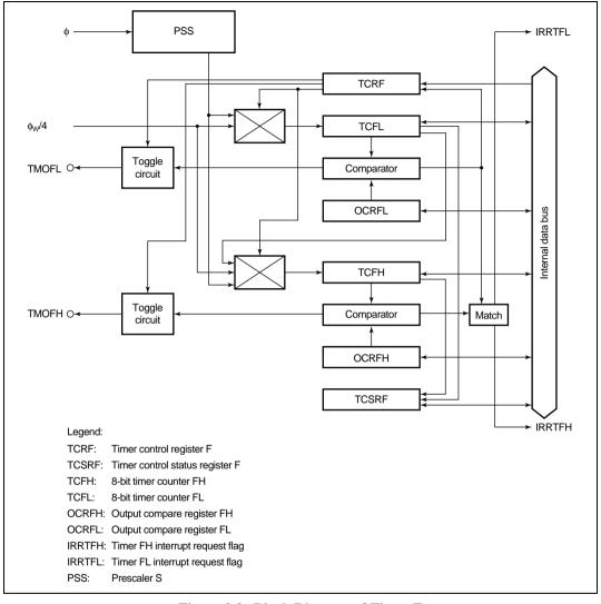
Figure 9.2 Block Diagram of Timer F
