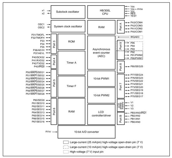
Figure 1.1 Internal Block Diagram of H8/3802 Group
