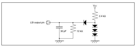
Figure 17.6 Output Load Circuit
