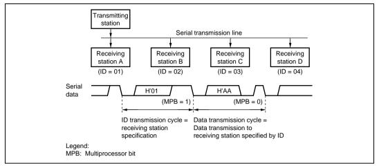
Figure 10.15 Example of Communication Using Multiprocessor Format (Transmission of Data H'AA to Receiving Station A)
