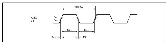
Figure 17.1 Clock Input Timing
