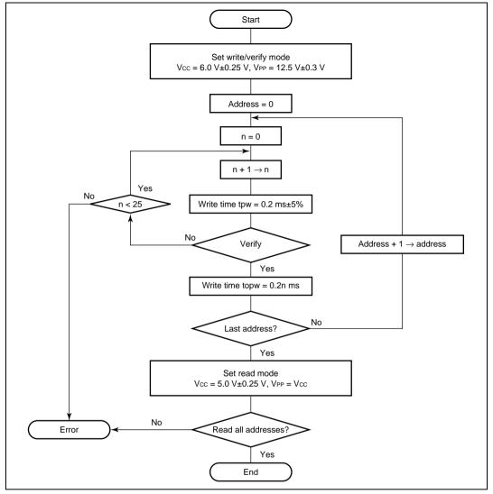
Figure 6.4 High-Speed, High-Reliability Programming Flowchart
