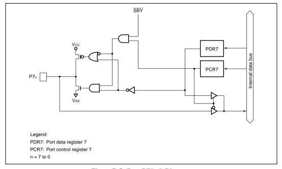
Figure B.5 Port 7 Block Diagram
