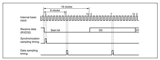
Figure 10.20 Receive Data Sampling Timing in Asynchronous Mode
