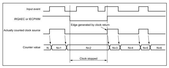
Figure 9.11 Example of Clock Control Operation
