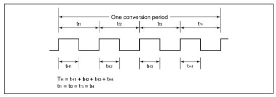
Figure 11.2 Waveform Output by 10-Bit PWM
