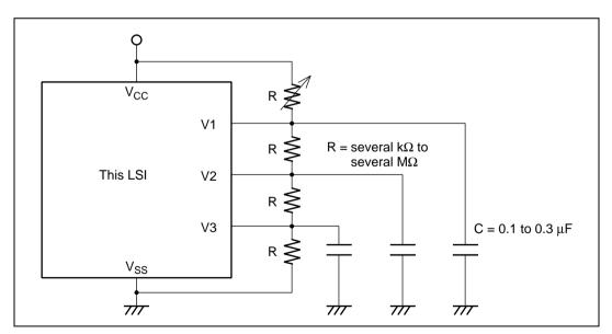
Figure 13.9 Connection of External Split-Resistance
