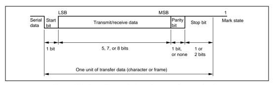
Figure 10.2 Data Format in Asynchronous Communication
