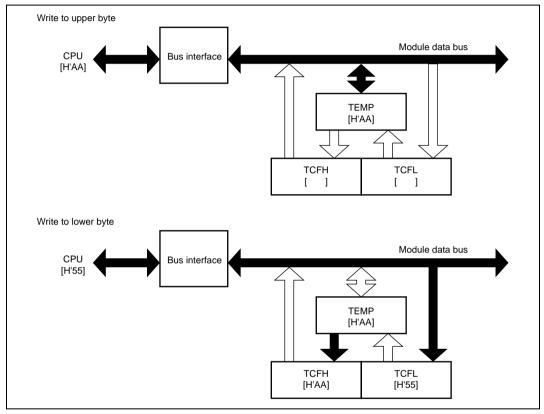
Figure 9.3 Write Access to TCF (CPU  $\rightarrow$  TCF)
