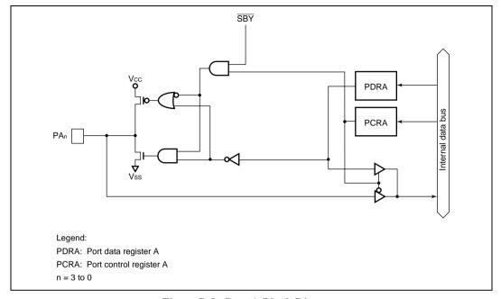
Figure B.8 Port A Block Diagram
