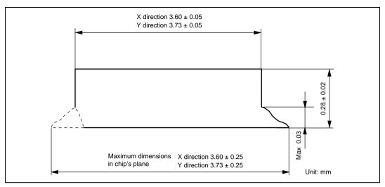
Figure F.1 Cross-Sectional View of Chip (HCD6433802, HCD6433801, and HCD6433800)
