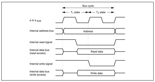
Figure 2.12 On-Chip Memory Access Cycle
