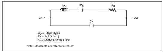
Figure 4.10 Equivalent Circuit of 32.768-kHz/38.4-kHz Crystal Resonator
