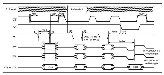
Figure 6.17 Timing Waveforms in Auto-Program Mode
