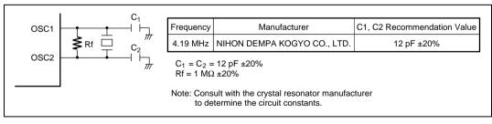
Figure 4.4(1) Typical Connection to Crystal Resonator (H8/3802 Group)
