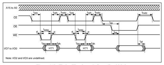
Figure 6.19 Timing Waveforms in Status Read Mode
