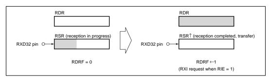
Figure 10.19(a) RDRF Setting and RXI Interrupt
