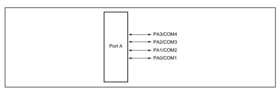
Figure 8.9 Port A Pin Configuration
