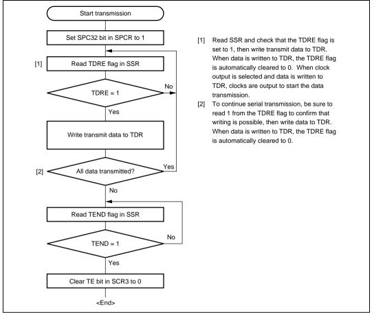
Figure 10.11 Sample Serial Transmission Flowchart (Clocked Synchronous Mode)
