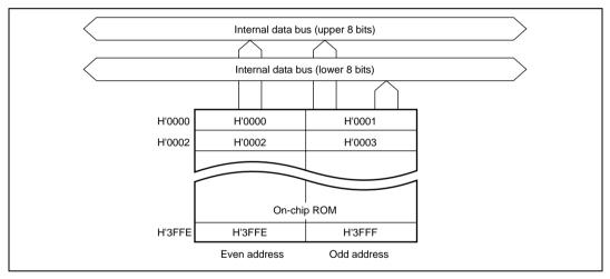
Figure 6.1 Block Diagram of ROM (H8/3802)
