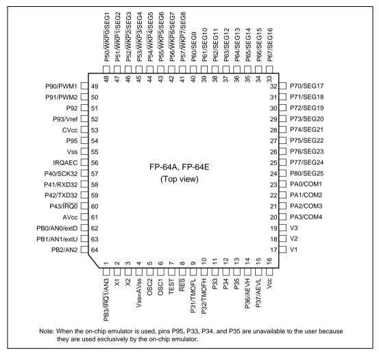
Figure 1.6 Pin Arrangement of H8/38104 Group (FP-64A, FP-64E)
