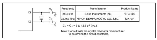
Figure 4.9 Typical Connection to 32.768-kHz/38.4-kHz Crystal Resonator
