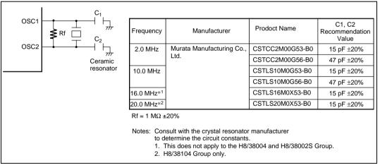
Figure 4.6(2) Typical Connection to Ceramic Resonator (H8/38004, H8/38002S, H8/38104 Group)
