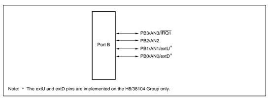
Figure 8.10 Port B Pin Configuration
