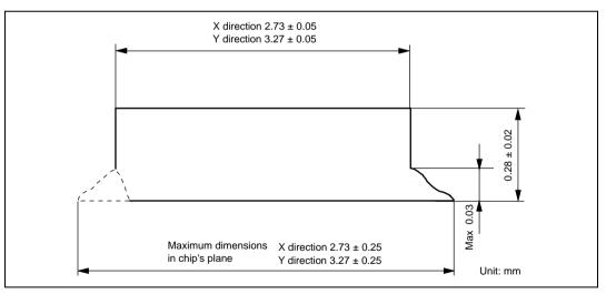
Figure F.2 Cross-Sectional View of Chip (HCD64338004, HCD64338003, HCD64338002, HCD64338001, and HCD64338000)
