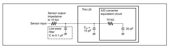
Figure 12.7 Example of Analog Input Circuit
