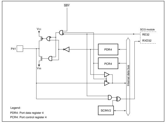
Figure B.2(c) Port 4 Block Diagram (Pin P41)
