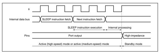
Figure 5.2 Standby Mode Transition and Pin States
