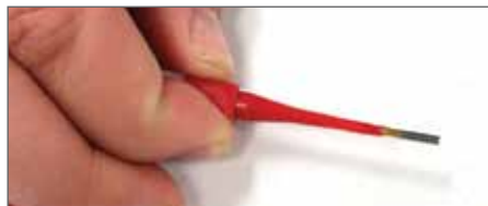
Plastic tool with contact in proper position.
