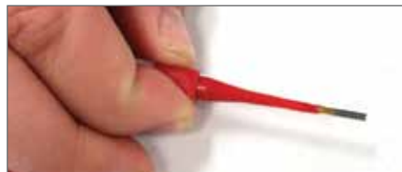
Plastic tool with contact in proper position.
