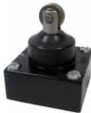
**LSD - Top roller plunger:** A corrosion-resistant steel roller and plunger that is adjustable to 90° angles to accept cam or slide operation from any of two directions. Boot seal on the plunger. Momentary action
