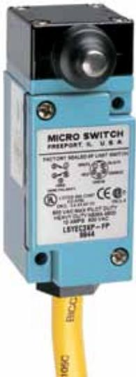
**Fully potted MICRO SWITCH™ HDLS heavy-duty limit switches** provide an extra degree of protection in harsh environments by sealing the basic switch cavity with epoxy. These switches are the same as the non-plug-in HDLS except that the entire switch cavity is filled with epoxy in addition to the conduit entrance. The fully potted HDLS switches are pre-ledged, with either cable or connectors.
