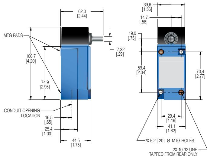
**Figure 3. MICRO SWITCH™ HDLS side rotary (double pole) dimensions**
