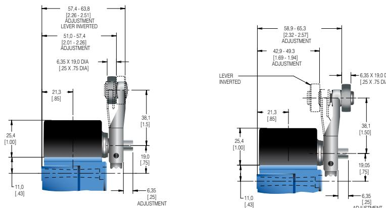
**Figure 7. LSZ52 type levers cam tracking**
