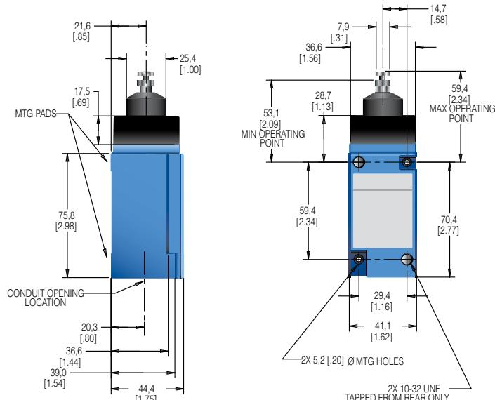
**Figure 15. MICRO SWITCH™ HDLS LSV Series top adjustable plunger (double pole) dimensions**
