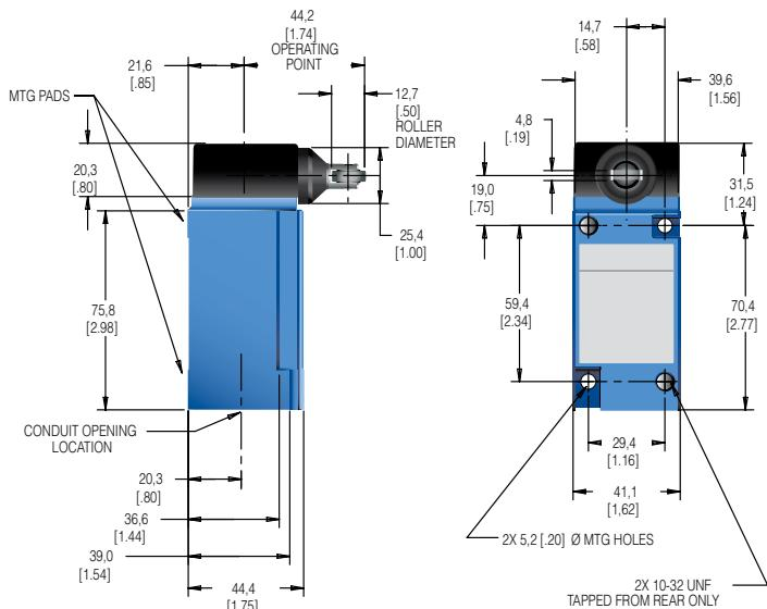
Figure 19. MICRO SWITCH™ HDLS LSF Series side roller plunger (double pole) dimensions
