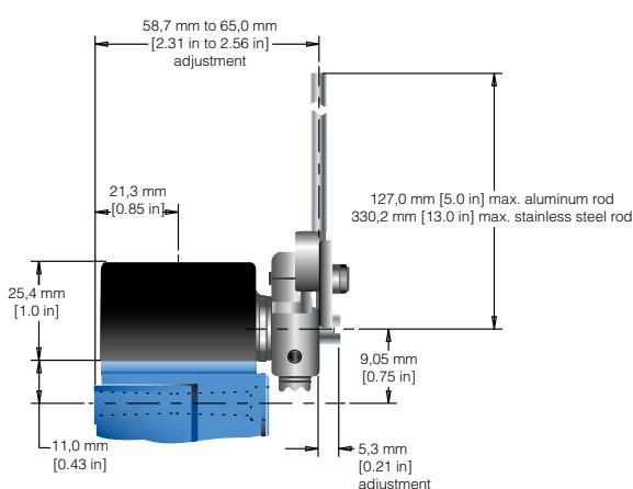
**Figure 9. LSZ55 type levers cam tracking**
