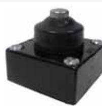
**LSC - Top pin plunger:** A corrosion-resistant steel plunger for in-line actuating motion. Oil-tight seals on plunger and between the operating head and housing keep out coolant, dust, and chips. Momentary action.
