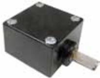
**LSA - Standard:** 60° minimum overtravel, 15° maximum pretravel, 5° (single pole) and 7° (double pole) maximum differential travel. Operating temperature range from -12 °C to 121 °C [10 °F to 250 °F].\*
