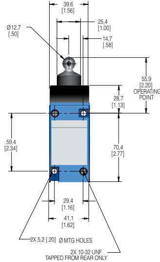
Figure 13. MICRO SWITCH™ HDLS LSD Series (double pole) top roller plunger dimensions
