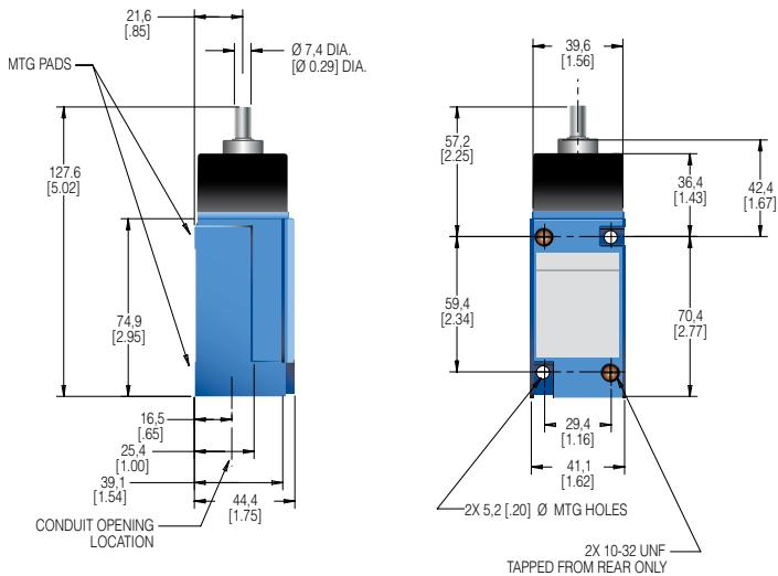
Figure 5. MICRO SWITCH™ HDLS top rotary (double pole) dimensions
