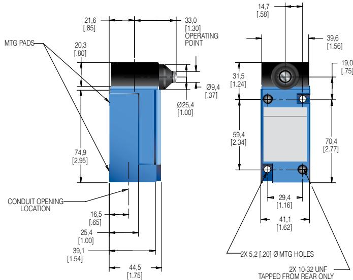
**Figure 17. MICRO SWITCH™ HDLS LSE Series side plain plunger (double pole) dimensions**
