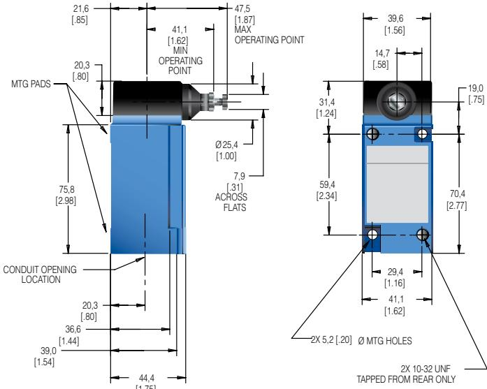
**Figure 21. MICRO SWITCH™ HDLS LSW Series side adjustable plunger (double pole) dimensions**
