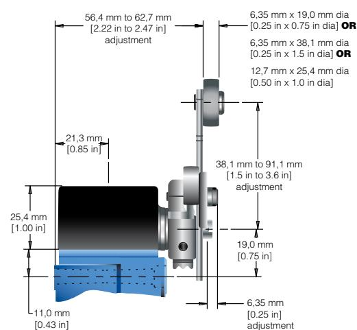
**Figure 8. LSZ54 type levers cam tracking**
