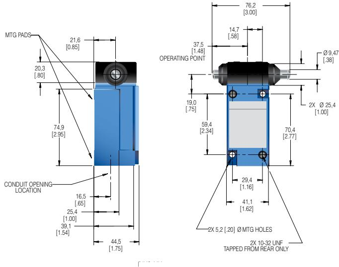
Figure 23. MICRO SWITCH™ HDLS LSG Series maintained contact side plunger (double pole) dimensions
