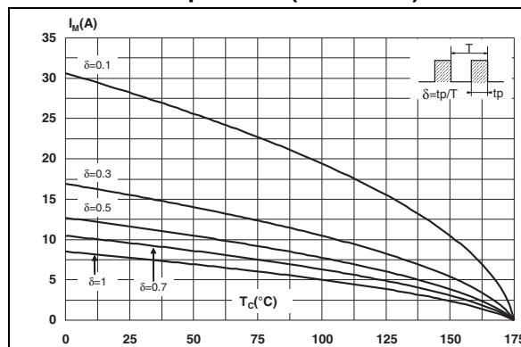
**Figure 4. Peak forward current versus case temperature (DPAK)**
