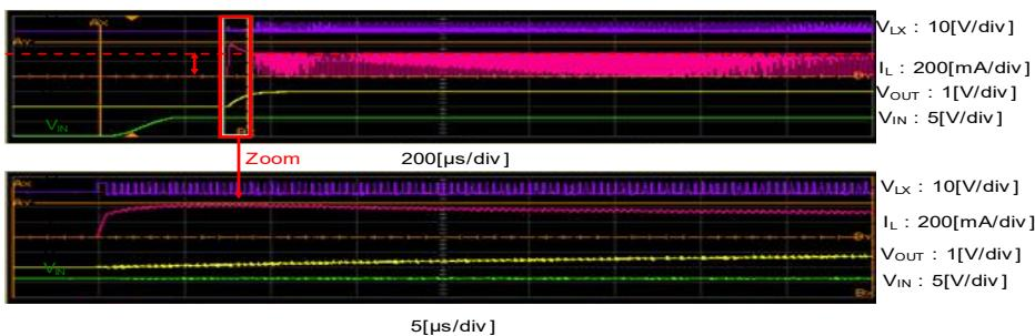
13. When the IC is started, the short-circuit protection function does not operate during the interval until the  $V_{OUT}$  voltage reaches a value near the set voltage.
