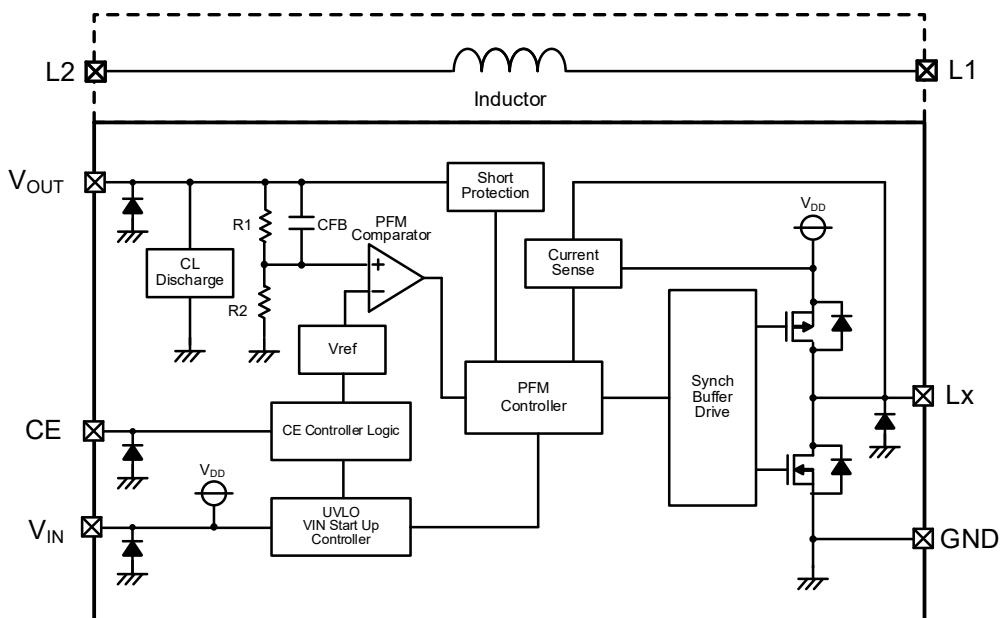
\* Diodes inside the circuits are ESD protection diodes and parasitic diodes.
