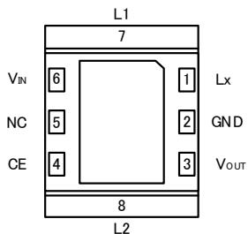
\* The dissipation pad for the CL-2025-02 package should be solder-plated in recommended mount pattern and metal masking so as to enhance mounting strength and heat release.
