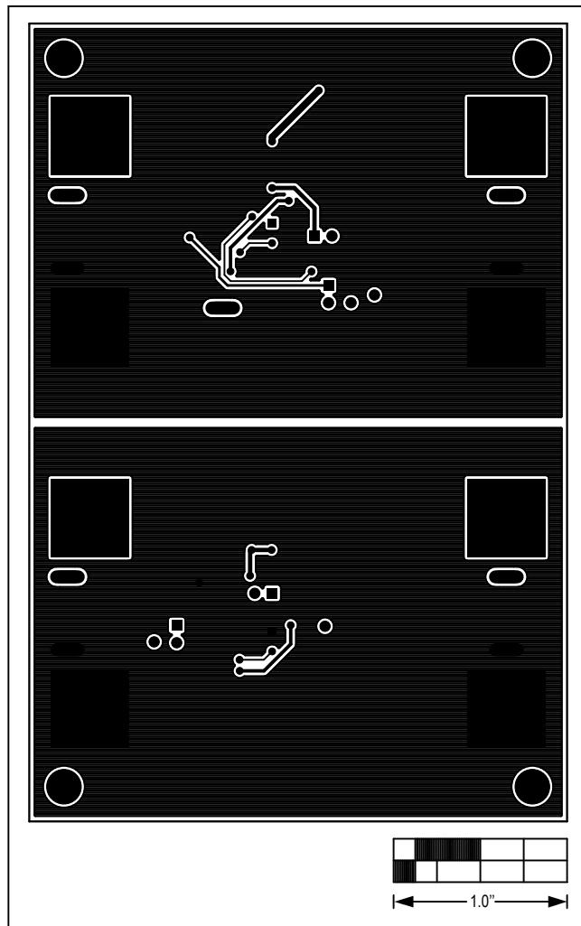
Figure 4. MAX16126/MAX16127 EV Kit PCB Layout—Solder Side
