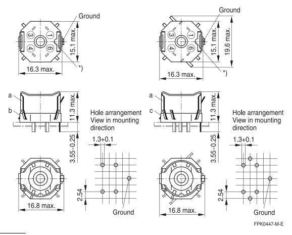
\*) This recess must be on the side of the grounding pin to ensure that the yoke locks in position.
