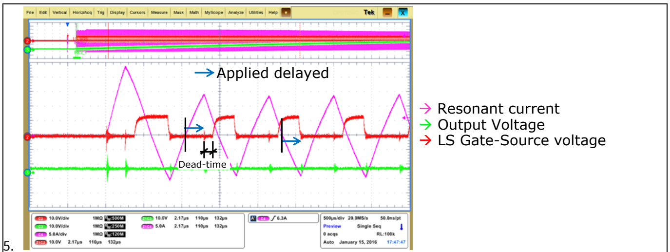
5. 6. Figure 27 LS-HS driving signal change is applied with a delay after the resonant current crosses zero to guarrante current polarity change and avoid hard-conmuation.
